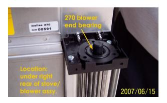
2. Remove the rubber end bearing carrier with thumb and forefinger by pulling on it.
