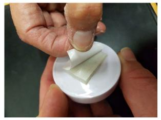
Remove the tape backing from Velcro if you want to mount the sensor (optional).
