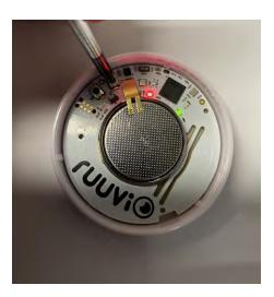
When mode button **B** is pushed both indicator lights shine bright
